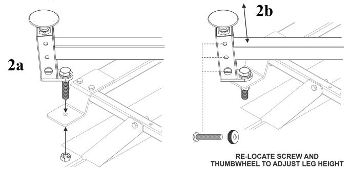
Carefully place the chair upright by reversing the procedure in '1'. The raiser is now fitted and ready for
