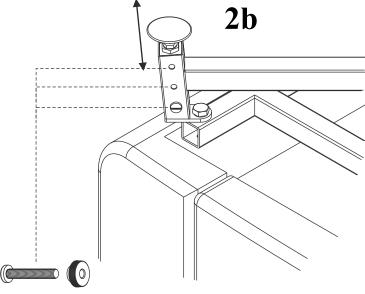
RE-LOCATE SCREW AND THUMBWHEEL TO ADJUST LEG HEIGHT
