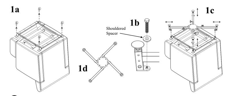
Position the square plate centrally to the legs and then tighten all the hand wheels. Secure the raiser using the supplied M6 nyloc nuts in all four positions (fig 2a). Adjust legs to required height and secure using height adjustment screw and thumbwheel (fig 2b).
