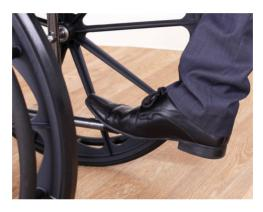
The attendant/carer then pushes the wheelchair forward and lifts the rear of the wheelchair up onto the kerb.
