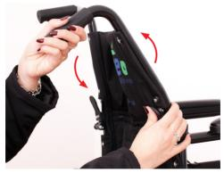
Repeat on the paddle on the other side. To return the backrest to the upright position, simply push the two handles back up into the upright position until the backrest locks in place.
